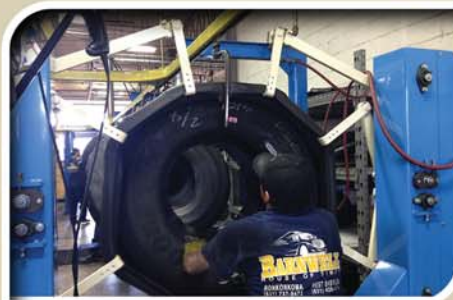
Technician places envelope around tire. Envelope must be connected to the EPS line. Tire is sent into curing chamber.
