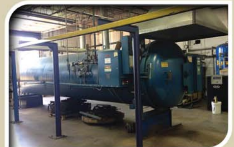
Technician places envelope around tire. Envelope must be connected to the EPS line. Tire is sent into curing chamber.
