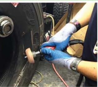
Technician will course buff area, wire brush and then apply "Black Cement".
