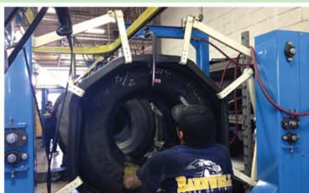
Technician places envelope around tire. Envelope must be connected to the EPS line. Tire is sent into curing chamber.
