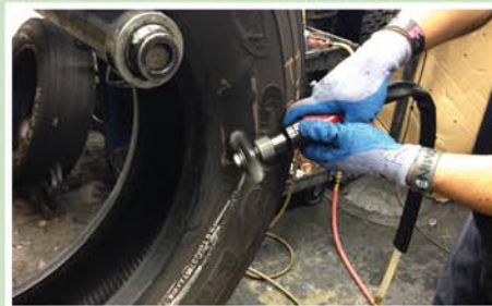
Technician will course buff area, wire brush and then apply "Black Cement".
