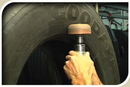
Use low speed buffer; buff area to "velvet-like" texture.
