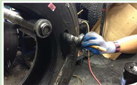
Technician will course buff area, wire brush and then apply "Black Cement".
