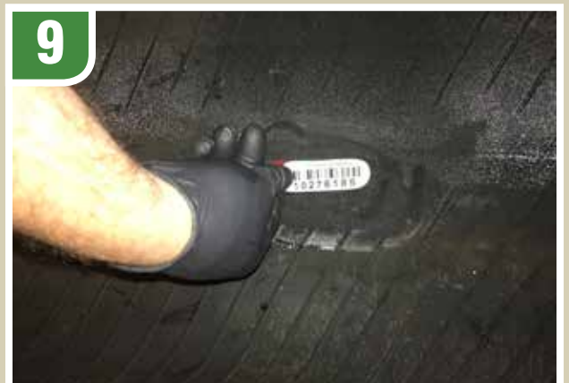
9 Place and Press ID UNIT in Cemented area.
