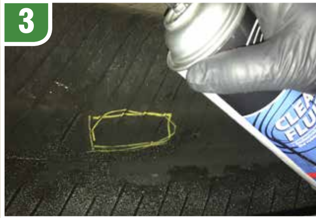
3 Spray area with Tire Cleaner Fluid and allow to penetrate.
