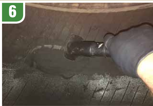
6 Vacuum or Wire Brush area to remove buffings.
