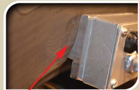
ID UNIT should be under lower curved section of contour plate.
