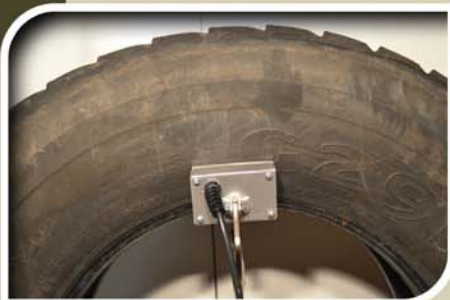
Lock HC onto tire so that it's extremely tight to the tire. HC should be “square” on tire.
