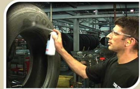
Spray with Tire Cleaning Fluid and allow to penetrate for 1 minute.
