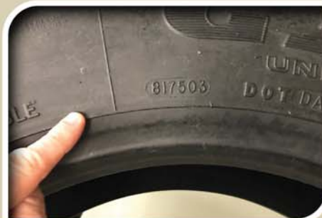
ID UNIT should be placed next to the D.O.T#. It should touch the “GG Ring”.
