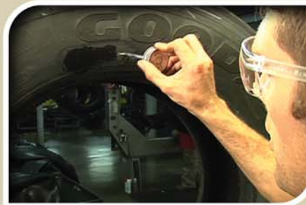
Apply thin coat of cement .
