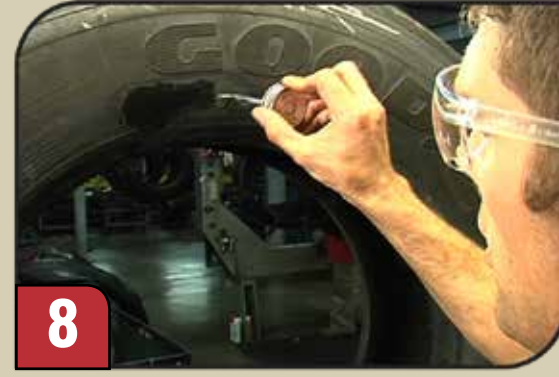
Apply thin coat of cement.
