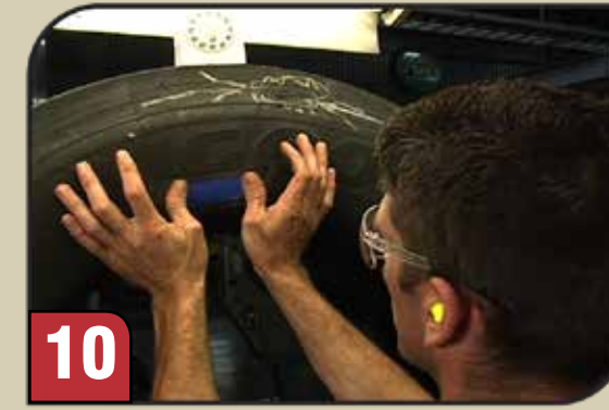
Place Primer Gum on tire. Press and smooth out with thumbs.
