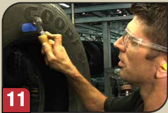
Remove tape and stitch roll to remove any trapped air.
