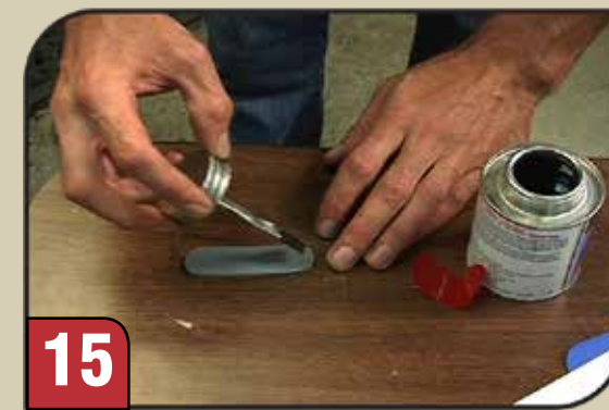
Apply thin coat of cement .
