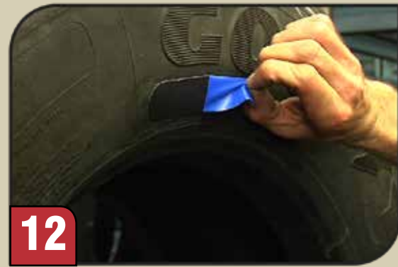
Peel back blue liner.
