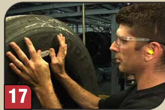
Place ID Unit on Primer Gum. Press and smooth out with thumbs.
