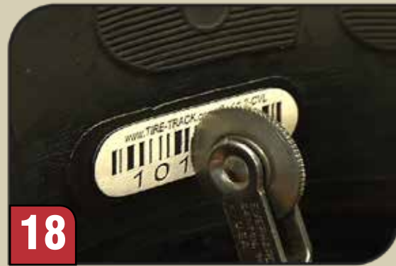
Stitch roll ID UNIT to remove any trapped air.
