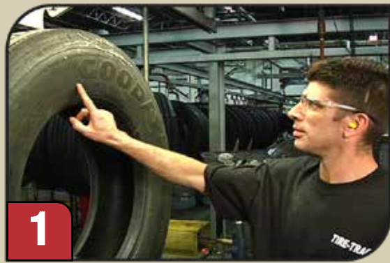
ID UNIT should be placed on the DOT side of the tire, touching the "GG Ring".
