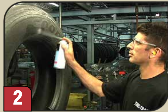
Spray with Tire Cleaning Fluid. Allow to penetrate and partially evaporate.
