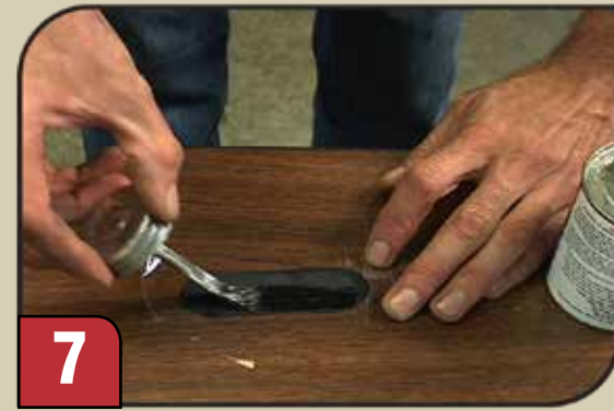
Remove "Blue Liner" and apply thin coat of cement.
