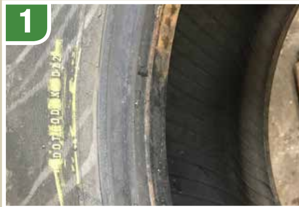
1 ID UNIT should be placed across from DOT#, on the INSIDE of the tire.
