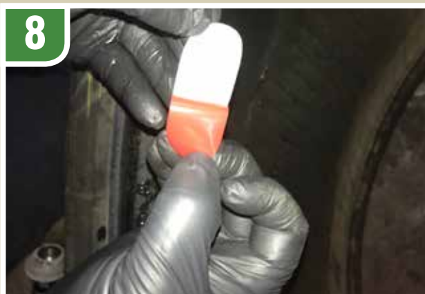
8 Remove backing from ID UNIT.
