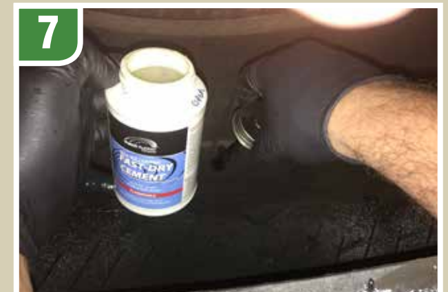
7 Apply PRC Chemical Vulcanizing Cement and allow to dry.
