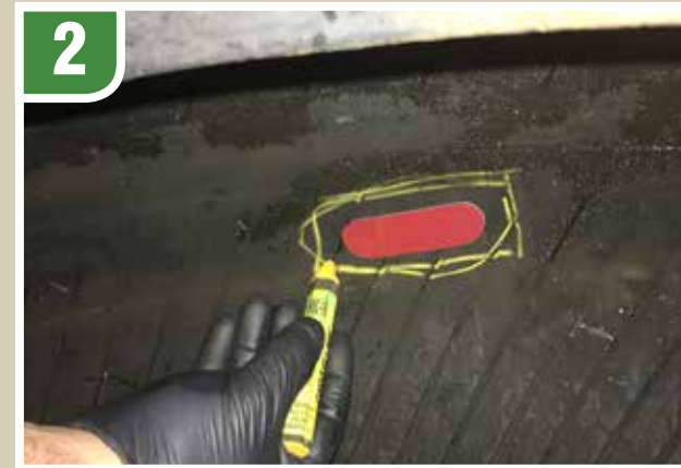
2 Place ID UNIT on the tread area and draw circle around ID UNIT with marker.
